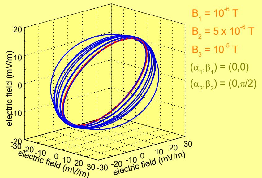
⇒ Retrieved THz-wave electric field ( $E_x = 15.88(92) \text{ mV/m}$ ,  $E_y = 15.74(72) \text{ mV/m}$ ,  $E_z = 15.831(3) \text{ mV/m}$ ,  $\phi_x = 0.78(6) \text{ rad}$ ,  $\phi_y = 1.05(1) \text{ rad}$ )
