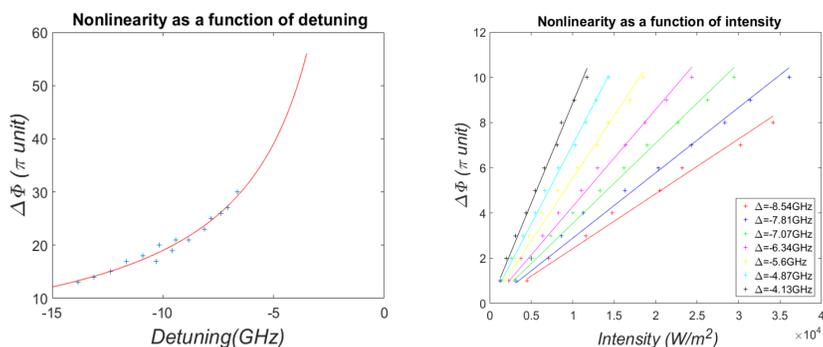
**Figure 2.** Left plot represents the non-linear phase-shift  $\Delta\phi$  as a function of the laser detuning. Right plot represents  $\Delta\phi$  as a function of the intensity.
